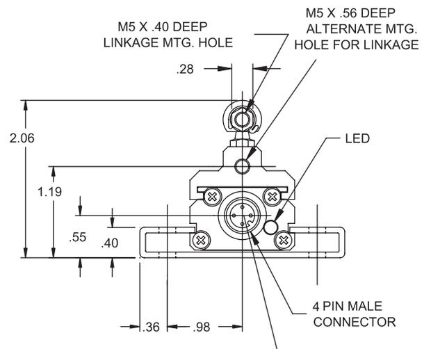
A standard 12 mm 4 pin micro connector is used. Straight mating cables can be ordered in a 6' length, or 12' length. If space is a consideration a right angle connector is also available.
