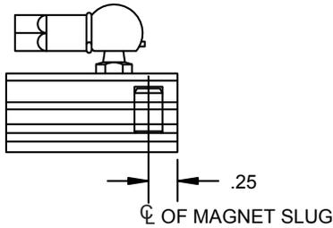
A standard female swivel mounting arm is provided with the slide magnet assembly. For extensions and other options contact the factory.
